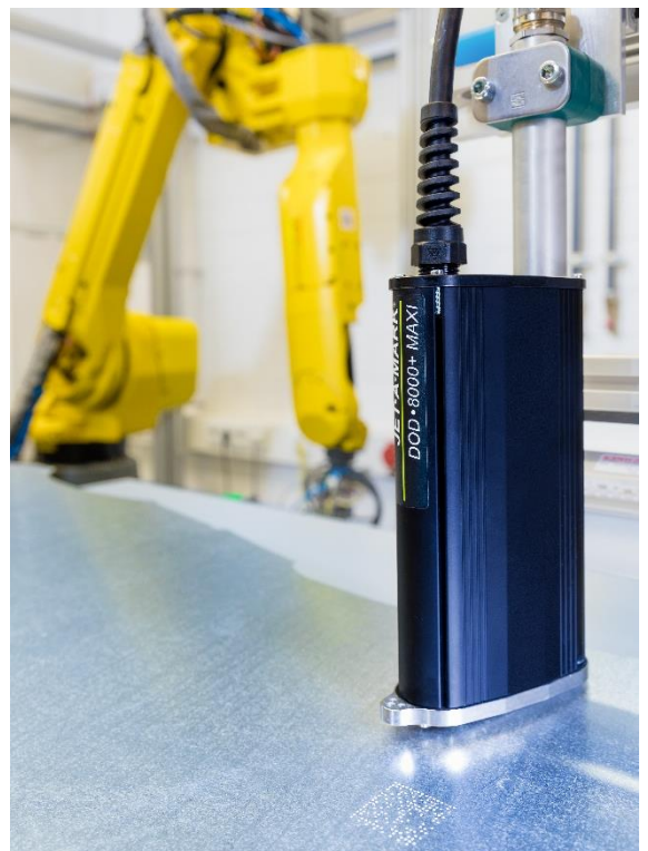
All in one system for an automated part marking
